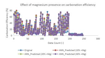
Figure 6. Carbonation efficiency with change in % of magnesium
