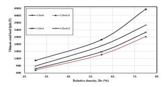
Figure 15. Relationship between ultimate axial Qult (N) load and relative dense, Dr (%)in different position of necking.
