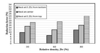
Figure 13. Relationship between axial compression load reduction factor (%) and relative displacement (Dr), in different positions of necking.
