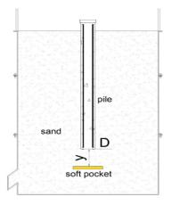
Figure 5. The details of the position of the soft pocket.
