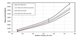
Figure 16. Relationship between ultimate axial Qult (N) load and relative dense, Dr (%) in different position of soft pocket.
