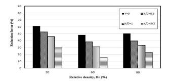
Figure 14. Relationship between axial compression load reduction factor (%) and relative displacement (Dr), in different positions of the soft pocket.
