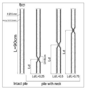
Figure 2. The details of defective and intact piles.
