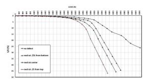
**Figure 9.** Relationship between axial compression load and relative displacement, S/D (%) for the sound pile and different defective model piles in the dense sand (Dr= 80%).
