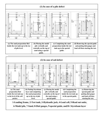
Figure 6. Installation steps for the defective sand and the pile.
