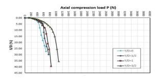
**Figure 10.** Relationship between axial compression load and relative displacement, S/D (%) for a pile based on soft pocket with different positions (Dr=30%).
