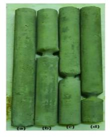
Figure 3. Model piles with different positions of neck.
