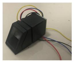
Figure 2. R305-optical fingerprint module
