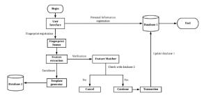
Figure 7. Software Architecture for Fingerprint based school debit transaction system
