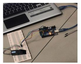
Figure 3. Fingerprint module connected to Arduino UNO board
