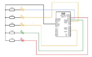
Figure 5. Circuit Diagram of the LED Indicators and Arduino UNO Board
