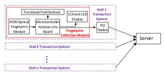
Figure 1. Fingerprint Recognition School Debit Transaction System
