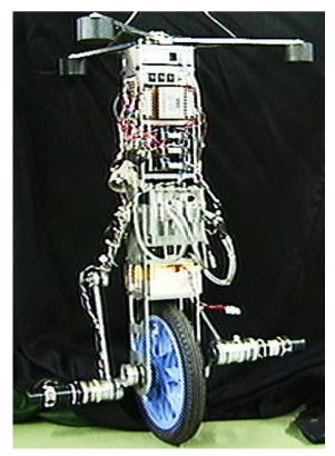
Figure 6. Robotic Unicycle model
