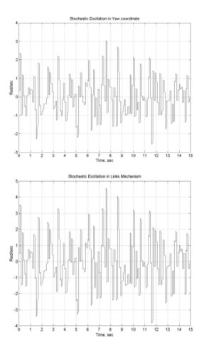
Figure 7. Simulated stochastic excitations - from a floor roughness's and jamming in closed-links mechanisms
