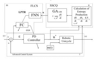
**Figure 3.** Self-organizing structure of an artificial intelligent (AI), robust control system design with a new physical measure of control quality
