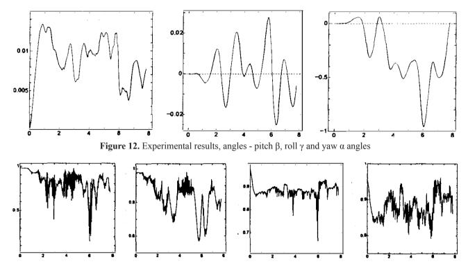
Figure 13. Experimental results of the fuzzy gains temporal behavior kp1, kd2, kp2, kd2 for 2 PD controllers
