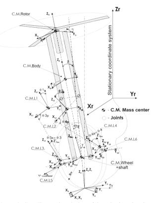
Figure 2. Coordinates description of the robotic unicycle model
