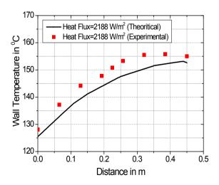
**Figure 6.** Theoretical result for wall temperature comparison with experimental for L/D=10
