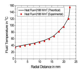
**Figure 7.** Theoretical result for fluid temperature comparison with experimental for L/D=18.89
