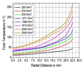
**Figure 5.** Theoretical result for fluid temperature for L/D= 18.89
