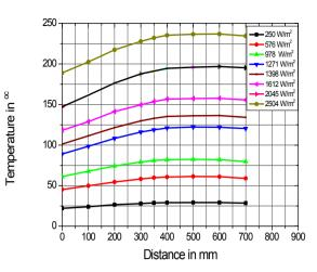
Figure 2. Wall temperature for various heat fluxes for (a) L/D ratio 10 and (b) L/D ratio 18.89
