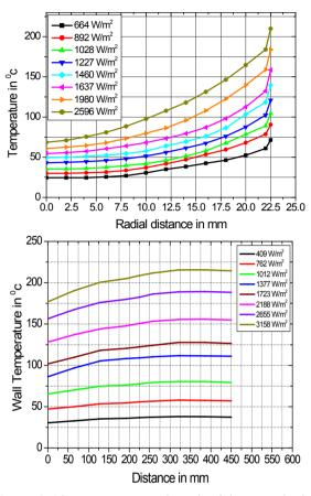
**Figure 4.** Air temperature at the exit of the smooth pipe with protrusions (L/D = 15.56, t = 4 mm, s = 283.33mm)
