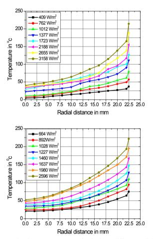
**Figure3.** Air temperatures at exit of tube at different radial distances for smooth tubes for (a) L/D ratio10 and (b) L/D ratio 18.89
