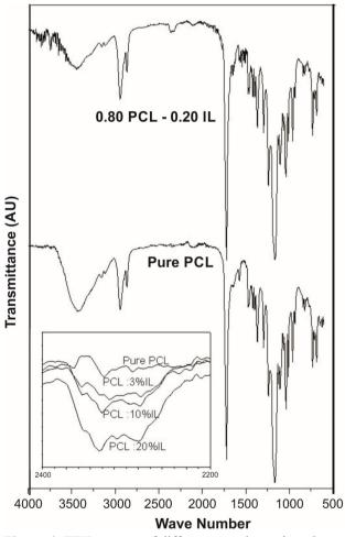
Figure 4. FTIR spectra of different constituent in polymer composite membrane
