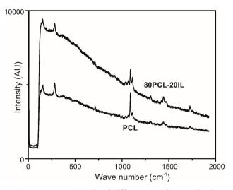
Figure 5. Raman Study of different constituent of polymer composite membrane
