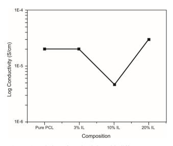
Figure 6. Variation of conductivity with different IL composition in polymer composite
