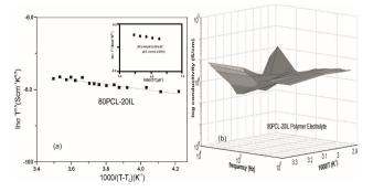
Figure 7(a). Variation of  $\ln \sigma$  with Temperature and (b): variation of conductivity with frequency and temperature in polymer composite membrane
