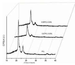
Figure 2. XRD spectra of the PCL and different PCL+IL composite system
