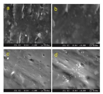
Figure 3. SEM image of (a) & (b) PCL membrane, (c) & (d) 80PCL-20IL electrolyte at two Magnifications
