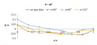
**Figure 20.** Bed variation of Bend 3, at angular displacement  $\theta = 40^{\circ}$  along the transverse direction when dyke installed at location 2,  $\theta = 40^{\circ}$
