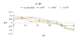
**Figure 18.** Bed variation of Bend 3 at angular displacement  $\theta = 80^{\circ}$  along the transverse direction when dyke installed at location 1,  $\theta = 0^{\circ}$
