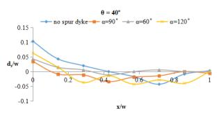
Figure 17. Bed variation of Bend 3 at angular displacement  $\theta = 40^{\circ}$  along the transverse direction when dyke installed at location 1,  $\theta = 0^{\circ}$
