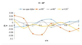
Figure 11. Bed variation of Bend 1, at angular displacement  $\theta = 40^{\circ}$  along the transverse direction when dyke installed at location 2,  $\theta = 40^{\circ}$
