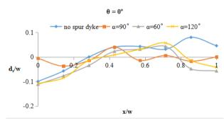
**Figure 16.** Bed variation of Bend 3 at angular displacement  $\theta = 0^{\circ}$  along the transverse direction when dyke installed at location 1,  $\theta = 0^{\circ}$
