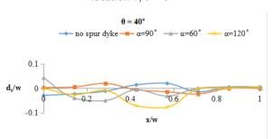
Figure 8. Bed variation of Bend 1 at angular displacement  $\theta = 40^{\circ}$  along the transverse direction when dyke installed at location 1,  $\theta = 0^{\circ}$
