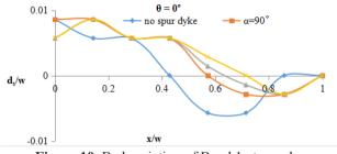
**Figure 10.** Bed variation of Bend 1 at angular displacement  $\theta = 0^{\circ}$  along the transverse direction when dyke installed at location 2,  $\theta = 40^{\circ}$
