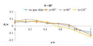
Figure 21. Bed variation of Bend 3 at angular displacement  $\theta = 80^{\circ}$  along the transverse direction when dyke installed at location 2,  $\theta = 40^{\circ}$
