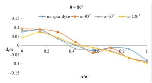
**Figure 12.** Bed variation of Bend 1 at angular displacement  $\theta = 80^{\circ}$  along the transverse direction when dyke installed at location 2,  $\theta = 40^{\circ}$
