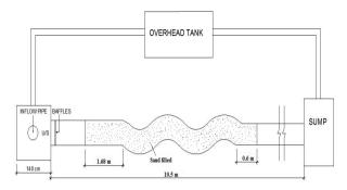
Figure 1. Schematic line diagram of bed flume
