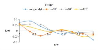
Figure 15. Bed variation of Bend 1 at angular displacement  $\theta = 80^{\circ}$  along the transverse direction when dyke installed at location 3,  $\theta = 60^{\circ}$
