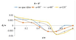
**Figure 13.** Bed variation of Bend 1 at angular displacement  $\theta = 0^{\circ}$  along the transverse direction when dyke installed at location 3,  $\theta = 60^{\circ}$
