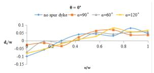
**Figure 22.** Bed variation of Bend 3 at angular displacement  $\theta = 0^{\circ}$  along the transverse direction when dyke installed at location 3,  $\theta = 60^{\circ}$
