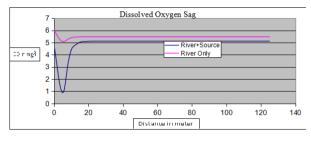
Figure 5. DO sag curve developed using Streeter Phelp's model (Shiroli MIDC)
