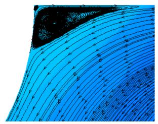
Figure 8. The streamlines bend vortex turbulator for a semicircular cross section with  $\text{Re} = 10^6$ ; d / D = 0,95 and d / D = 0,90; t / D = 0,50 for air, shown on a larger scale than in Figure 6
