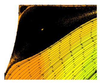
**Figure 5.** The flow lines for the angular vorticity of turbulizer semicircular cross section with  $\text{Re} = 10^6$ ; d / D = 0,95 and d / D = 0,90; t / D = 0,25 for air, shown on a larger scale than in Figure 3
