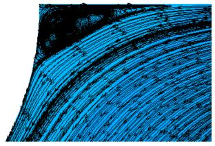
Figure 11. The streamlines bend vortex turbulator for a semicircular cross section with  $Re = 10^6$ ; d / D = 0,95 and d / D = 0,90; t / D = 1,00 for air, shown on a larger scale than in Figure 9
