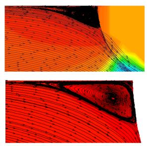
Figure 10. The streamlines bend vortex turbulator to semicircular cross-section with Re = 10+; d / D = 0,95 and d / D = 0,90; t / D = 1,00 for air, shown on a larger scale than in Figure 9
