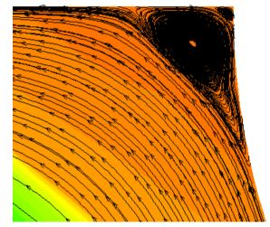
Figure 4. The flow lines of bend to vortex turbulator semicircular cross section with  $\text{Re} = 10^6$ ; d / D = 0,95 and d / D = 0,90; t / D = 0,25 for air, shown on a larger scale than in Figure 3
