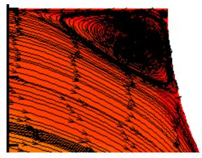
Figure 7. The flow lines of bend to vortex turbulator semicircular cross section with  $\text{Re} = 10^6$ ; d / D = 0,95 and d / D = 0,90; t / D = 0,50 for air, shown on a larger scale than in Figure 6
