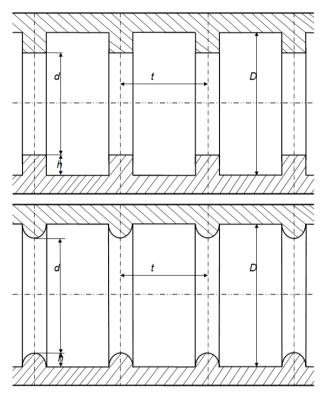
Figure 1. Cut a straight circular tube with a transverse surface located turbulators and flow square semicircular (lower panel) cross-sections
