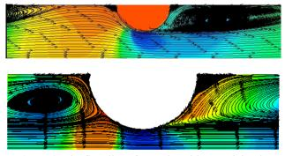
Figure 3. The flow lines for a tube with a semicircular cross-sectional turbulence at Re =  $10^6$ ; d / D = 0,95 and d / D = 0,90; t / D = 0,25 for air
