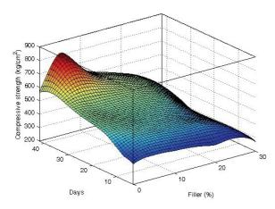
Figure 8. Predicted results of the comprehensive strength (kg/cm2) using ANN1
