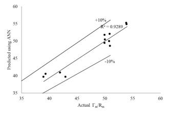
Figure 9. Actual v/s predicted results of the deformability and viscosity indices using ANN2
