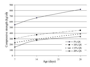
Figure 4. Compressive strength versus age (Mix QS+SF)
