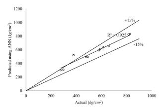
Figure 7. Actual v/s predicted results of the 28-day compressive strength(kg/cm<sup>2</sup>) using ANN1
