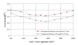
Figure 3. Void fraction of aggregates mixes, before and after compaction process
