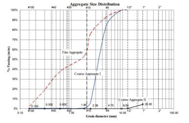
Figure 1. Sieve analysis of fine and two types of coarse aggregates
