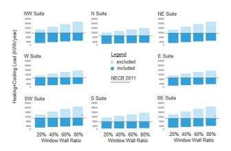
**Figure 4.** Range of combined heating and cooling loads for various windows to wall ratios by suite orientation
