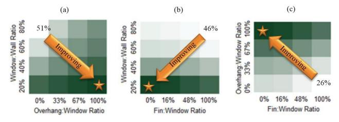
**Figure 9.** Qualitative trends in average net energy consumption for a) window to wall ratio vs. overhang to window ratio. b) fin to window ratio vs. overhang to window ratio, and c) overhang to window ratio vs. fin to overhang ratio
