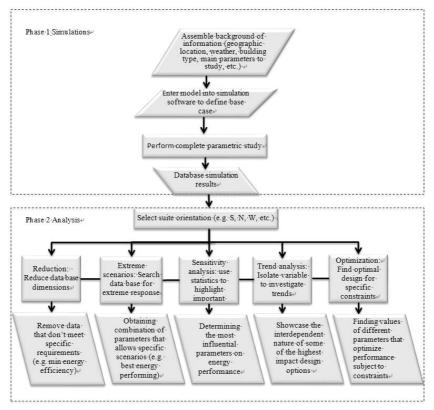
Figure 1. Design performance modelling workflow template
