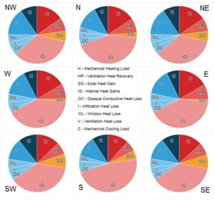
**Figure 5.** Response variables for lowest net energy scenario (heat losses in blues, heat gains in reds/orange)
