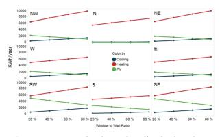
Figure 7. WWR vs heating and cooling loads and PV potential for eight suite types (all simulations)
