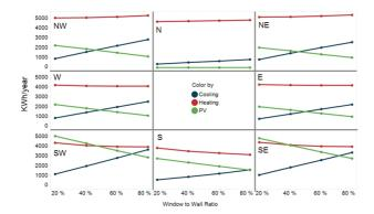
**Figure 8.** WWR vs heating and cooling load and PV potential for eight suite types with quadruple glazed, high SHGC windows
