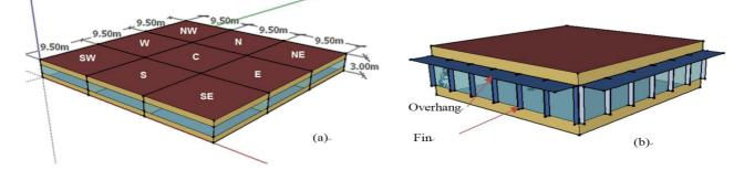
**Figure 2.** (a) Geometry of the eight unique suites of a story of the base case, and common area 'C'; (b) Illustration of the use of overhang and fins in the simulations.
