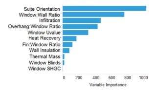
Figure 6. Relative impact of Input variable on net energy
