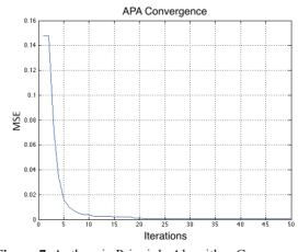
**Figure 7.** Anthropic Principle Algorithm Convergence stopping criterion: 100 iterations. In the GA, the crossover rate starting in 80% and ending with 60%, the mutation rate starting in 5% and ending in 10%. The resulting MSE of the approximated model provided by the APA and GA are given in table 5.
