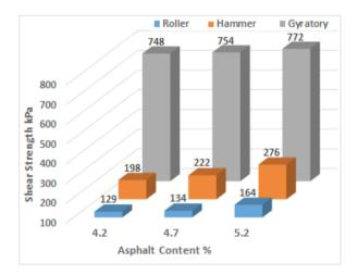
Figure 3. Influence of Binder Content on Shear Strength
