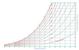
Figure 3. Air thermal process on psychometric chart
