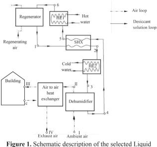
Figure 1. Schematic description of the selected Liquic Desiccant Cooling (LDC) system
