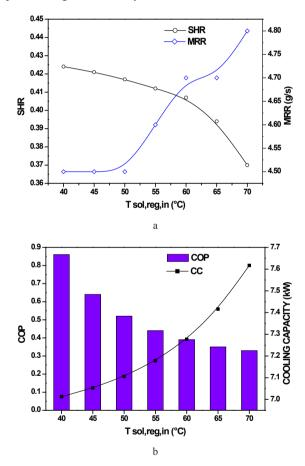
**Figure 7.** Influence of inlet desiccant solution temperature to the regenerator (Tsol,reg,in) on: a. SHR and MRR and b. the performance of the system
