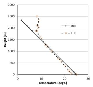
Figure 3. ABL Height determination using Parcel Method
