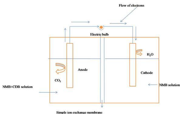
**Figure 3.** Dual chambered Microbial Fuel Cells (MFCs) Construction and Operation
