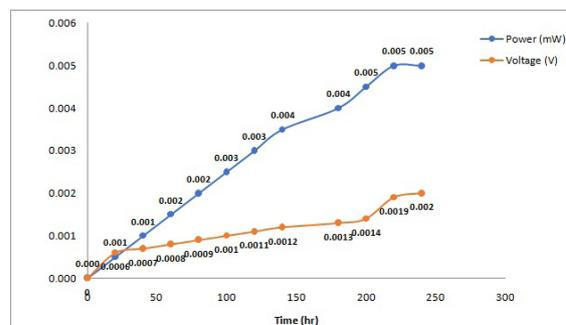
**Figure 5.** Generation of power corresponded with voltage from rice paddy straw
