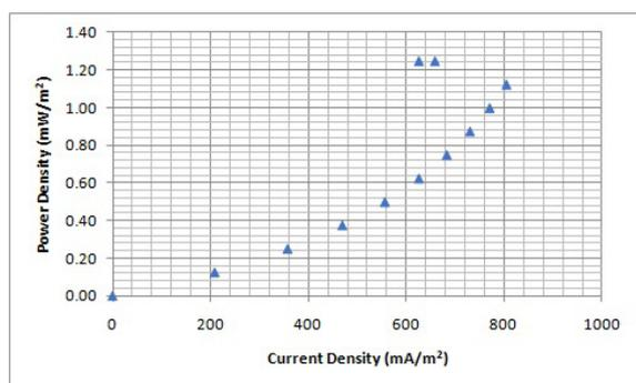
**Figure 7:** Power density versus Current density through rice paddy straw
