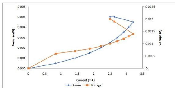
**Figure 6.** Polarization and power density curves through rice paddy straw
