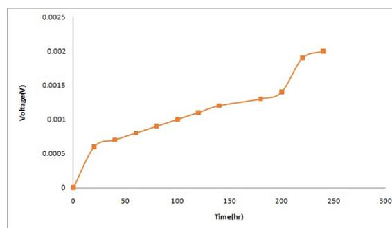
**Figure 4.** The generation of voltage through rice paddy straw at 1000Ω resistance
