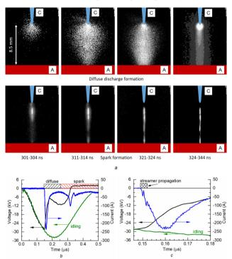
Figure 9. (a) ICCD images of a discharge in the point-to-plane gap filled with air at a pressure of 100 kPa. C – cathode, A – anode. (b, c) Waveforms of voltage and discharge current pulses. Negative polarity. Setup 2
