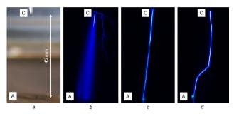
**Figure 6.** Image of the needle-to-plane gap and images of a discharge plasma emission. Setup 1. Negative polarity
