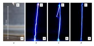
Figure 4. Image of the cone-to-plane gap and images of a discharge plasma emission. Setup 1. Negative polarity
