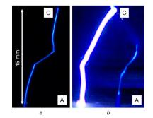
Figure 5. Images of the discharge plasma emission in the cone-to-plane gap. Setup 1. Negative polarity
