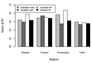
Figure 6. NASH criterion values and coefficient of determination by hydrologic station.
