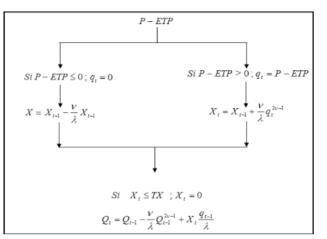
Figure 2. Schematic of the ModHyPMA model and key model equations <sup>[32,28,29]</sup>.
