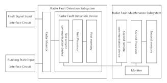
**Figure 1.** Icon Schematic diagram of fault maintenance system for new generation weather radar
