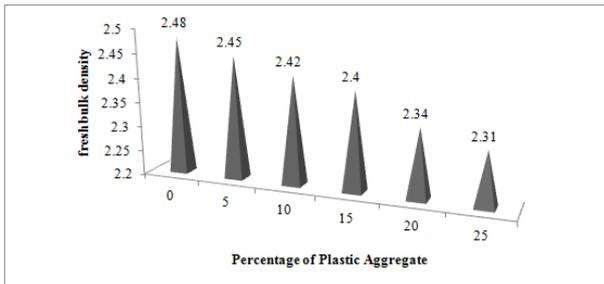
Figure 4.2 Density of Concrete Mixtures
