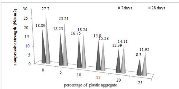
Figure 4.3 Compressive Strength of Concrete Mixtures
