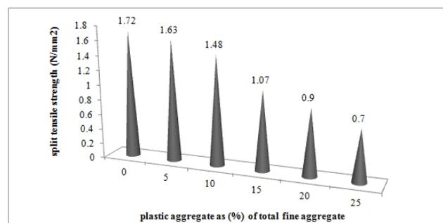
Figure 4.5 Split Tensile Strength of Concrete Mixtures
