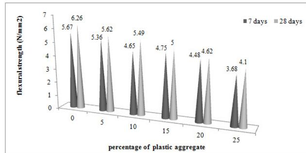
Figure 4.4 Flexural Strength of Concrete Mixtures
