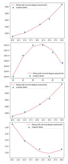
It can be obtained from the analysis of the diagram that when the ratio of powder distribution is 15-25, the assimilation temperature of sinter is higher and the liquid phase fluidity of sintered products is low, that is, the quality of sintered mineral products is relatively high and the energy consumption cost of sintering process is relatively low.
