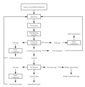
Figure 1. Typical sintering process
