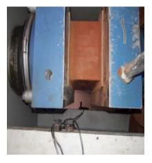
Figure 4. Compressive Strength test
