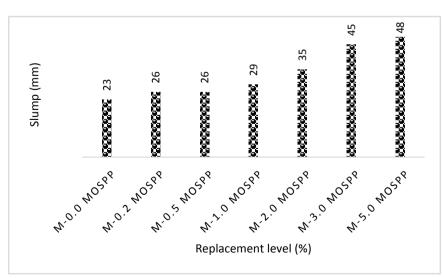
Figure 8. Slump of MOSP-Concrete
