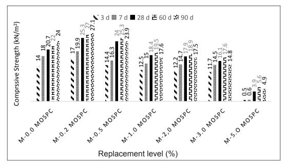
Figure 13. Compressive Strength of MOSP-Concrete
