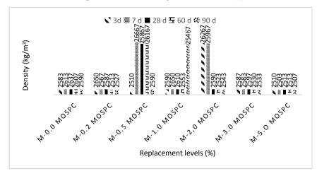
Figure 12. Density of MOSP-Concrete
