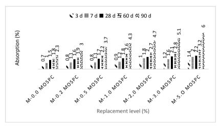
Figure 10. Water Absorption of MOSP-Concrete
