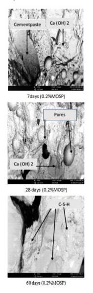
Figure 5. Micrograph of MOSP-Concrete
