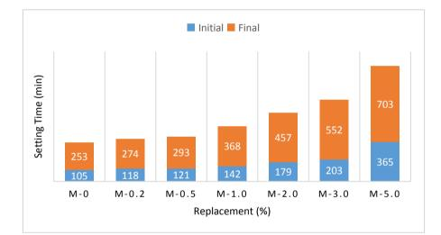
Figure 7. Setting Times of MOSP Cement Paste
