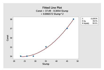
Figure 9. Consistency against the Slump
