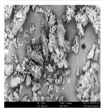
Figure 2. Microstructure of MOSP
