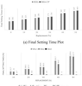
(b) Final Setting Time Difference Figure 6. Final Setting Time of RHA-CP-OPC Paste
