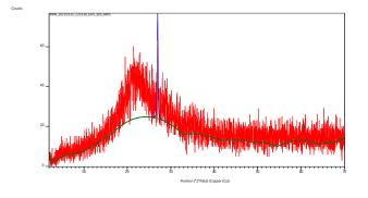
Figure 2. XRD Diffractograme of RHA
