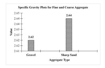
Figure 4. Specific Gravity Plots for both fine and coarse aggregates
