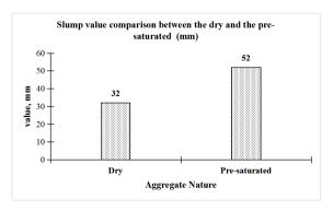
Figure 6. A Bar Chart Showing the Comparison between the Workability of the Dry and Pre-Saturated Coarse Concrete
