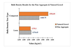
Figure 5. Bulk Density Plots for the Natural Gravel & Fine Aggregate
