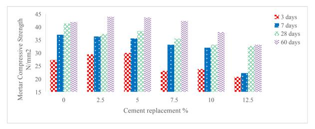
Figure 8. Effect of cement replacement on the mortar compressive strength of various cement blended BEPA and curing days
