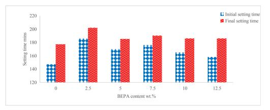
Figure 7. Effect of BEPA content on Setting times of cement blends
