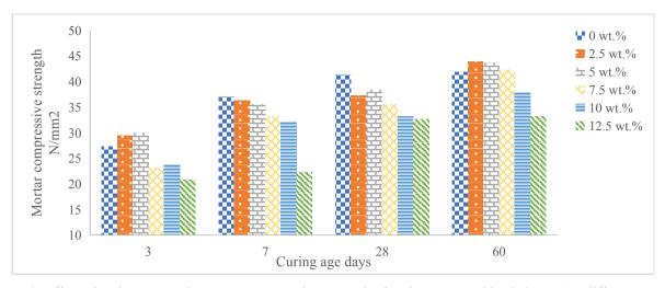
Figure 9. Effect of curing age on the mortar compressive strength of various cement blended BEPA at different cement replacements
