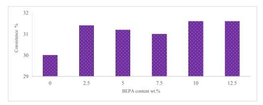
Figure 6. Effect of BEPA content on water consistence of cement blends
