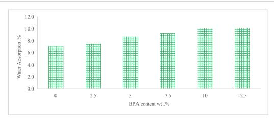
Figure 5. Effect of BEPA content on Water Absorption of cement blends
