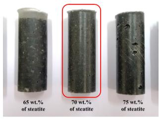
Figure 8. Polymer-based Composites with 65 wt.%, 70 wt.% and 75 wt.% of Steatite Inclusions
