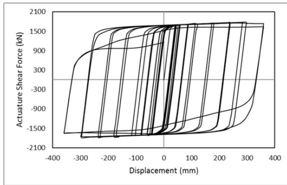
**Figure 10b.** Force-displacement Diagram under the Influence of Far Pattern (Frame With Buckling Restrained Brace)
