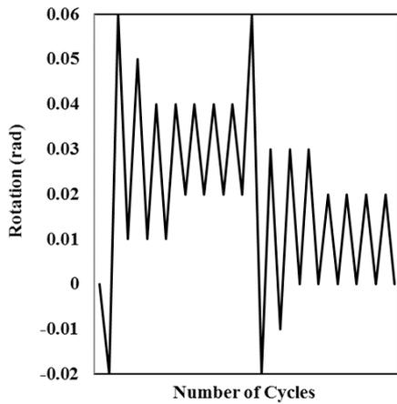
Figure 4a. Sac Cyclic Loading (Near Fault)
