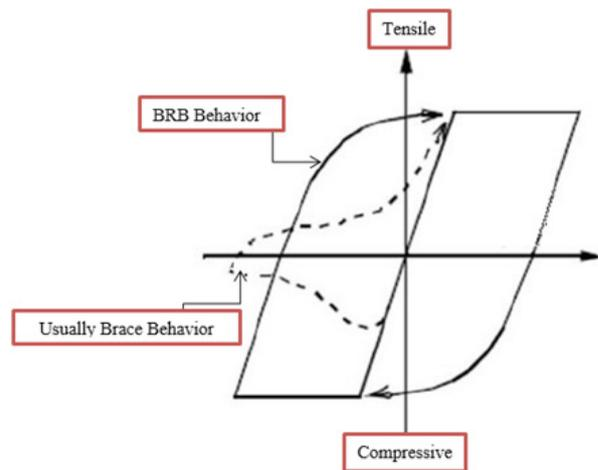
**Figure 1.** The Ideal Behavior of Buckling-restrained Brace<sup>[9]</sup>
