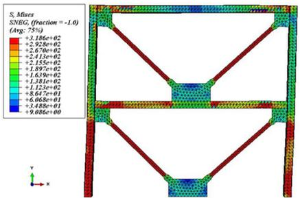
Figure 8b. Buckling Restrained Brace Stress Contour
