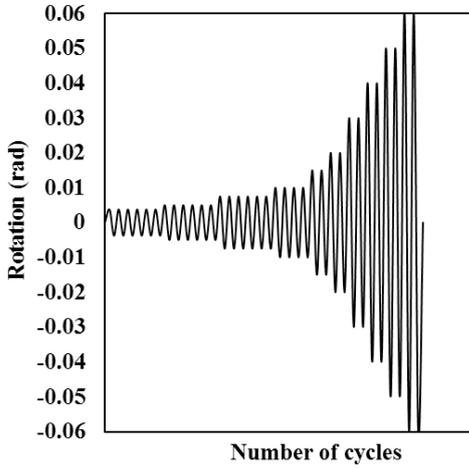
Figure 4a. Sac Cyclic Loading (Far Fault)
