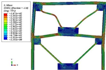
Figure 8a. Conventional Brace Stress Contour
