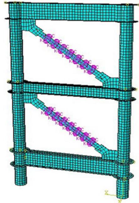
Figure 6. Numerical Model Constructed Based on Laboratory Model [14]
