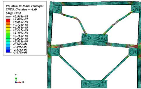
Figure 9a. Stress Contour of Conventional Brace
