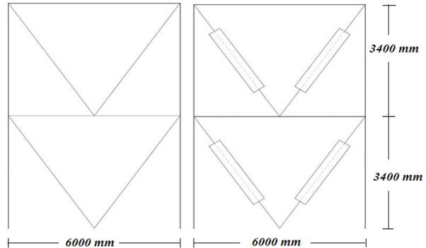
**Figure 3a.** Moment Frame Model with Conventional Chovern Brace (VCBF)
