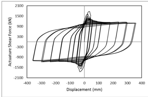
**Figure 10a.** Force-displacement Diagram under the Influence of Far Pattern (Frame with Conventional Brace)
