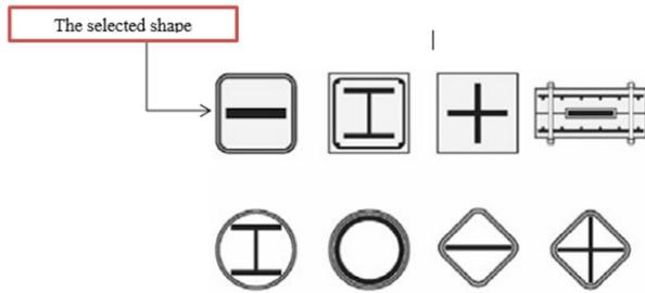
**Figure 2.** Variants of Buckling Restrained Braces
