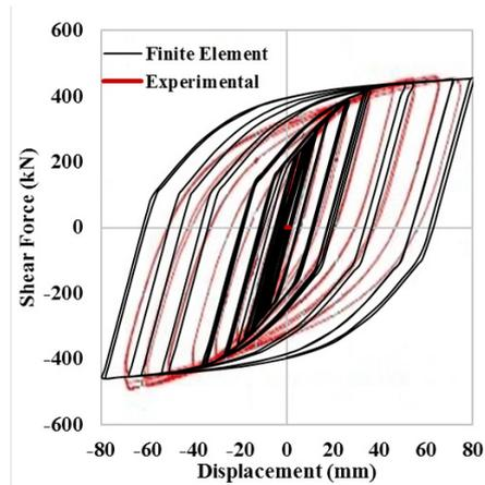
Figure 7. Comparison of Hysteresis Curves of the Numerical Model and Laboratory Samples
