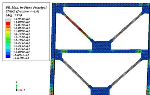
Figure 9b. Buckling Restrained Brace Stress Contour
