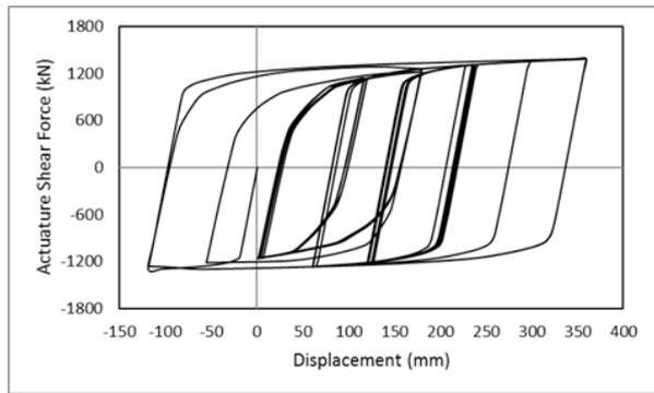
**Figure 11b.** Force-displacement Diagram under the Influence of Near Pattern (Frame with Buckling Restrained Brace)
