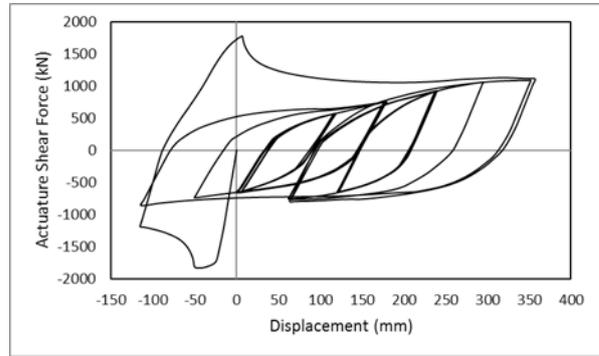
**Figure 11a.** Force-displacement Diagram under the Influence of Near Pattern (Frame with Conventional Brace)
