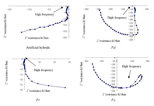
Figure 8. Impedance complex plane for artificial hybrids, Pinus densata (P.d), Pinus tabuliformis(P.t) and Pinus yunnanensis (P.y)
