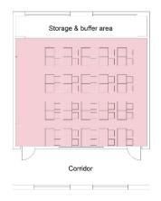
Figure 14. Plan of Classroom with Buffer Area at North to Support Improved Air Exchange
