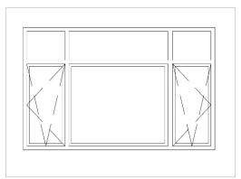
Figure 12: Profile of Tilt and Turn Windows
