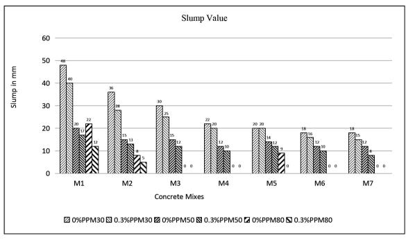
Figure 2. Graphical representation of slump test results
