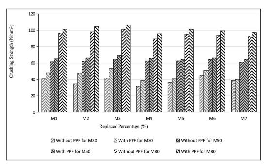
Figure 6. Graph showing Crushing strength of FS & CCW for 28 days curing
