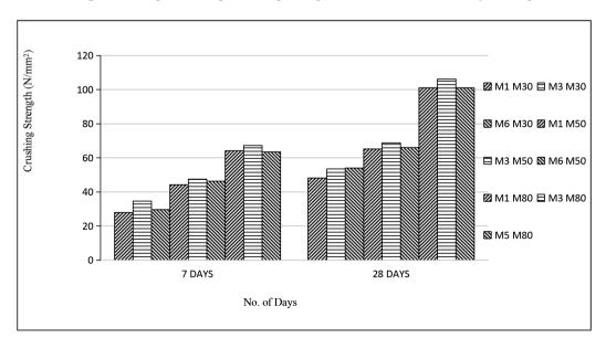
Figure 7. Graph showing Crushing strength of FS & CCW for 7 and 28 days curing
