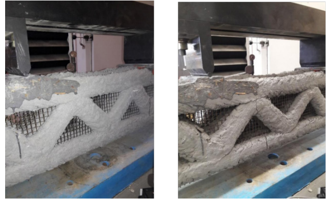
Figure 19. Basalt Mesh Beam Before and After Loading and Crack Propagation
