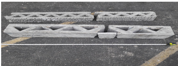
Figure 18. Failure of Printed (top) and Cast (bottom) Beams
