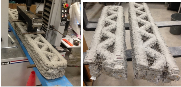
Figure 22. Printed Basalt Mesh Beam Before and After Lateral Loading
