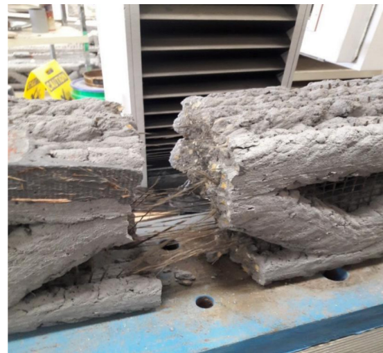
Figure 20. Basalt Mesh Splitting
