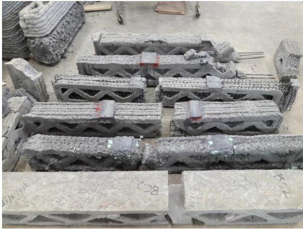
Figure 17. Six Types of Beams That Were Tested to Failure by Four Point Bending: Cast (bottom), Unreinforced, 0.64 cm Mesh, 2.54 cm Mesh, 0.95 cm Basalt Rebar, 0.95 cm Steel Rebar (top)
