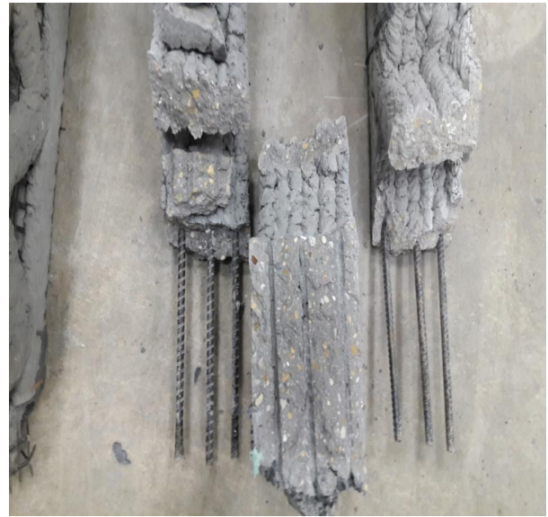
Figure 24. Break Site of Steel (left) and Basalt (right) Rebar
