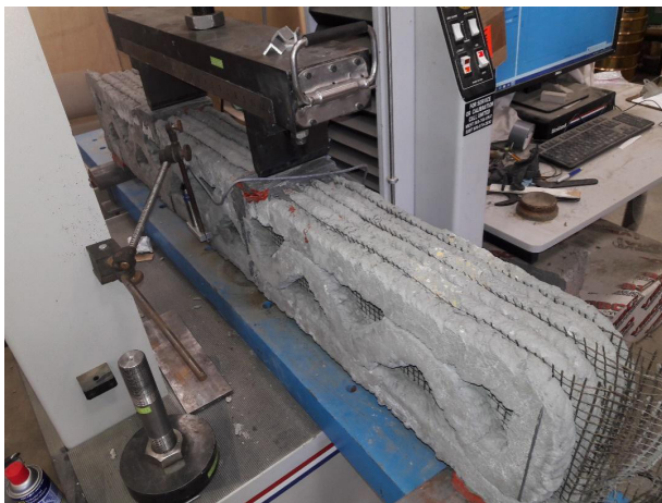
Figure 5. Test apparatus for Testing Printed Concrete Beams
