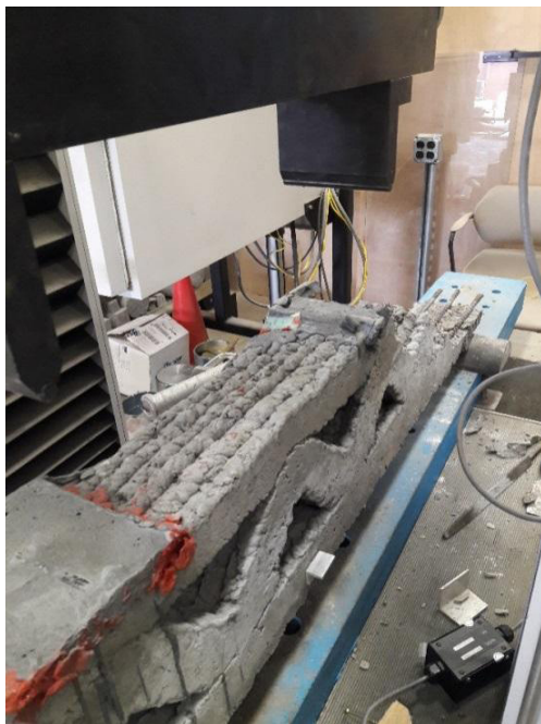
Figure 23. Failure of Rebar-Reinforced Concrete
