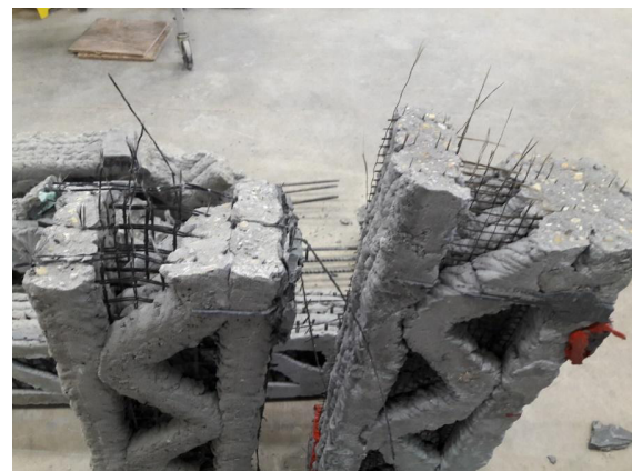
Figure 21. Break Site of Aramid (left) and Basalt (right) Mesh
