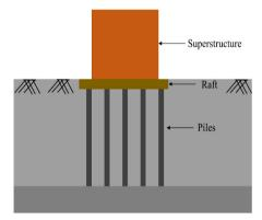
Figure 2. Piled raft foundation
