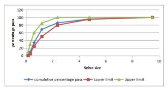
Figure 1. Gradation curve of fine aggregates by cumulative percentage pass
