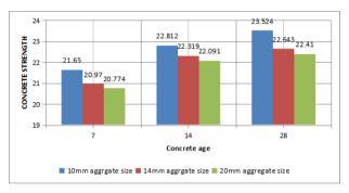
Figure 3. Compressive strength of concrete at different ages with different aggregate sizes
