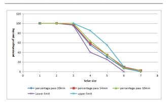
Figure 2. Gradation curves of coarse aggregate for 20mm, 14mm and 10mm by their percentage of passing
