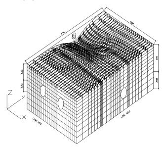
Figure 1. A case of shield tunneling ground settlement stimulated by 3-dimational finite element
