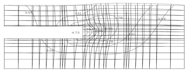
Figure 5. Longitudinal map of stratum deformation induced by shield tunneling
