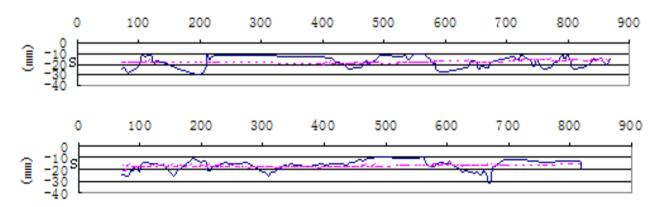
Figure 6. Two cases of ground deformation along with the longitudinal center of shield tunneling
