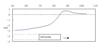
Figure 3. Longitudinal ground settlement induced shield tunneling
