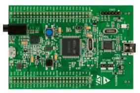
Figure 1. STM32F407VGTx microcontroller
