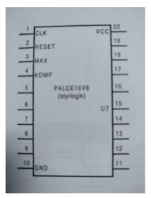
Figure 9. Configuration scheme of the control logic (PAL-CE16V8)
