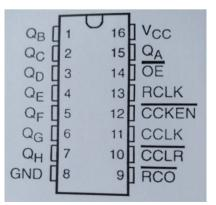
Figure 6. Configuration scheme of Synchronous counter, SN54HC590A
