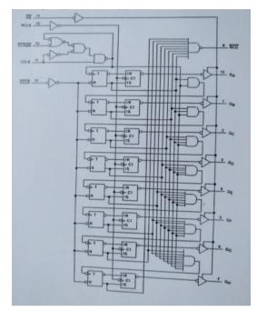
Figure 7. Map of the synchronous counter connecting lines
