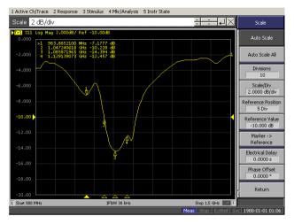
Figure 12. S11-value of the proposed tag antenna with L1 at 13.4 nH
