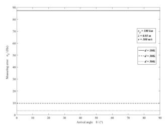
Figure 10. The measurement error of the change rate of Doppler at different baseline lengths
