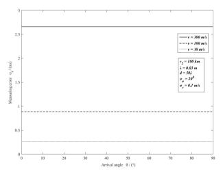
Figure 12. The measurement error at different flight speeds
