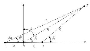
Figure 3. The one-dimensional double base array with three units
