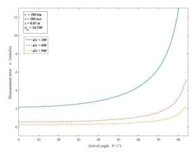
Figure 8. the angular velocity measurement error at different baseline lengths
