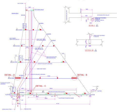
Figure 7. Maximum non-overflow section showing location of different instruments at PHEP-II dam (Ref: CWC/INST/ PNSC-9810-C-2131(R1))<sup>[7]</sup>
