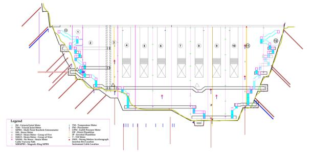
Figure 5. Longitudinal section at dam axis showing location of different instruments at PHEP-II dam (Ref: CWC/INST/ PNSC-9810-C-2132(R1))<sup>[7]</sup>
