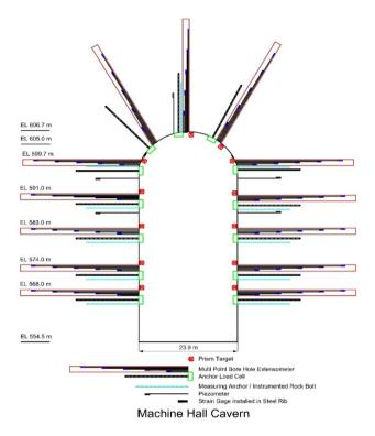
Figure 9. Section showing the location of different instruments in Machine Hall Cavern, PHEP-II<sup>[1][5][8]</sup>
