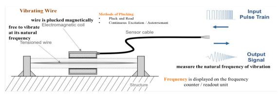
Calibration curve or table or linearizing circuit through **gage factors** are used for calculating desired parameter from change in frequency.
