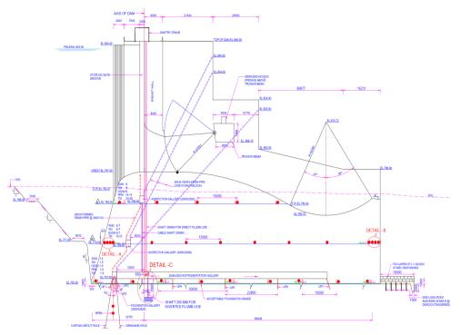
Figure 6. Maximum sluice section showing location of different instruments at PHEP-II dam (Ref: CWC/INST/PNSC-9810-C-2130(R1))<sup>[7]</sup>
