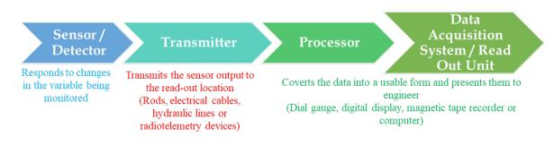
Figure 2. Components of an instrument
