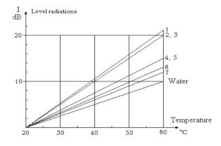
Figure 7. Dependence of radiation level of building materials on temperature
