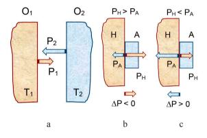
**Figure 3.** Distribution of energy flows between an arbitrary tangent objects: (a) – applicator and patient's body; b) negative energy flow; c) positive energy flow;
