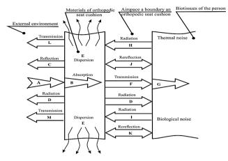
Figure 5. Model of interaction of electromagnetic currents at the material-human boundary
