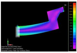
**Figure 7.** First run of the FEM with the 100 lbs load at the tip
