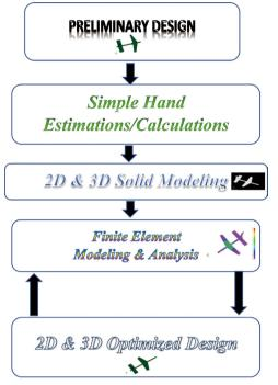
Figure 3. FEA Application for Design Iterations
