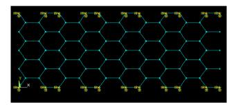
**Figure 4.** Free-Free-Clamp-Clamp (F-F-C-C) Boundary Condition (SFA)
