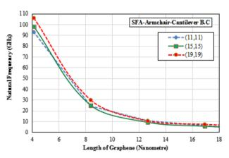
**Figure 9.** Variation of Natural Frequency in Cantilever Boundary Condition
