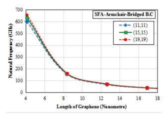
**Figure 8.** Variation of Natural Frequency in Bridged Boundary Condition
