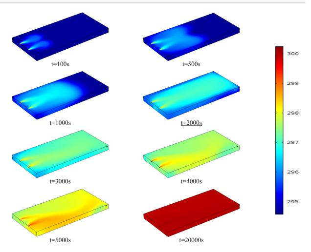
Figure 1. Temperature distribution during the injection process of warm water
