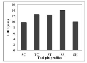
Figure 4. Effect of different tool pin profiles on the formability of the welded blanks
