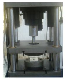
Figure 3. Arrangement of hydraulic press with punch, dies and welded blank
