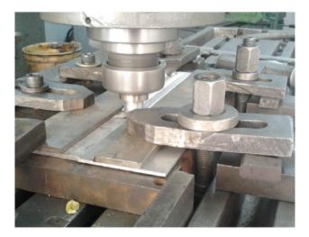
Figure 1. FSW arrangement
