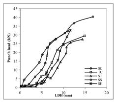
Figure 6. Punch load and limiting dome height diagram for welded blanks made with different tool pin profiles
