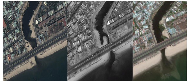
Figures 7a, b, and c. A river mouth with tidal inlet area much smaller than the width between constructed retaining walls
