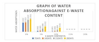
Figure 5. Variation of water absorption with E-waste content
