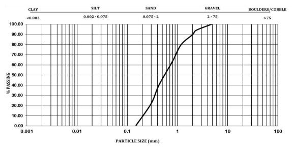
Figure 1. Variation of %Passing with sieve sizes for fine aggregate (sand)
