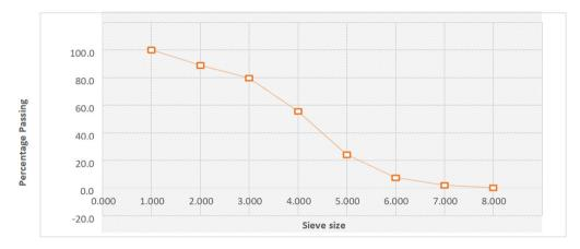
Figure 3. Variation of % Passing with sieve sizes for E-waste plastic
