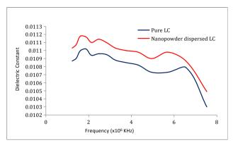
Figure 1. Variation of Dielectric Constant with frequency for pure and nanopowder dispersed LC
