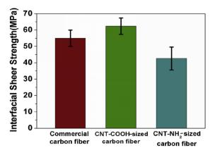
**Fig. 5.** Fragmentation tests for modified JH-T800 single-fiber composites. **Figure 2.** Fragmentation test for modified carbon fiber <sup>[11]</sup>
