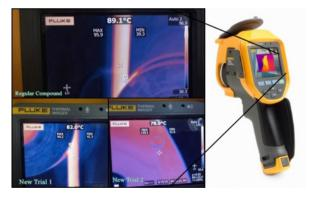
Figure 22. Belt Temperature Study by IR Thermal Imager
